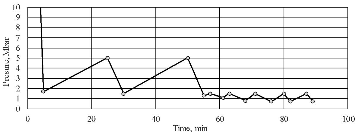
Fig. 1. Dynamics of pressure change at the first stage of the experiment in the freeze-dryer working chamber
